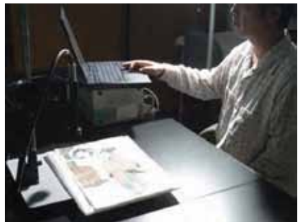
Figure 5: On-site analysis of color materials used for ukiyo-e prints by visible reflection spectroscopy
